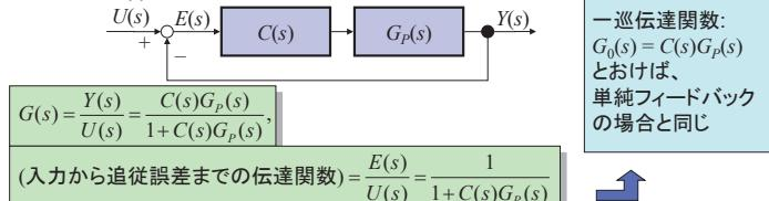
$$G(s) = \frac{Y(s)}{U(s)} = \frac{C(s)G_p(s)}{1 + C(s)G_p(s)}, \quad (\text{入力から追従誤差までの伝達関数}) = \frac{E(s)}{U(s)} = \frac{1}{1 + C(s)G_p(s)}$$
