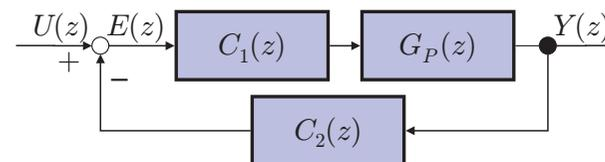
$$G(z) = \frac{Y(z)}{U(z)} = \frac{C_1(z)G_P(z)}{1 + C_1(z)C_2(z)G_P(z)}, \quad E(z) = \frac{1}{1 + C_1(z)C_2(z)G_P(z)}$$
